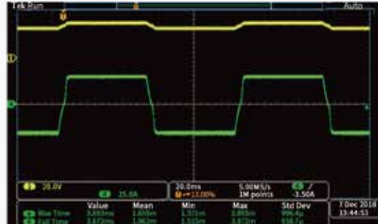
Control loop CC priority mode
